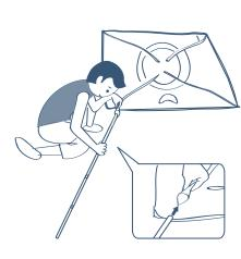
**STEP 4** Connect the poles to the base of each corner.
